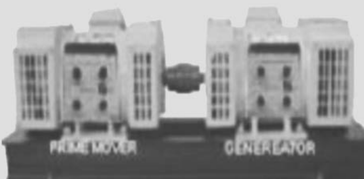
Motor Generator Set
